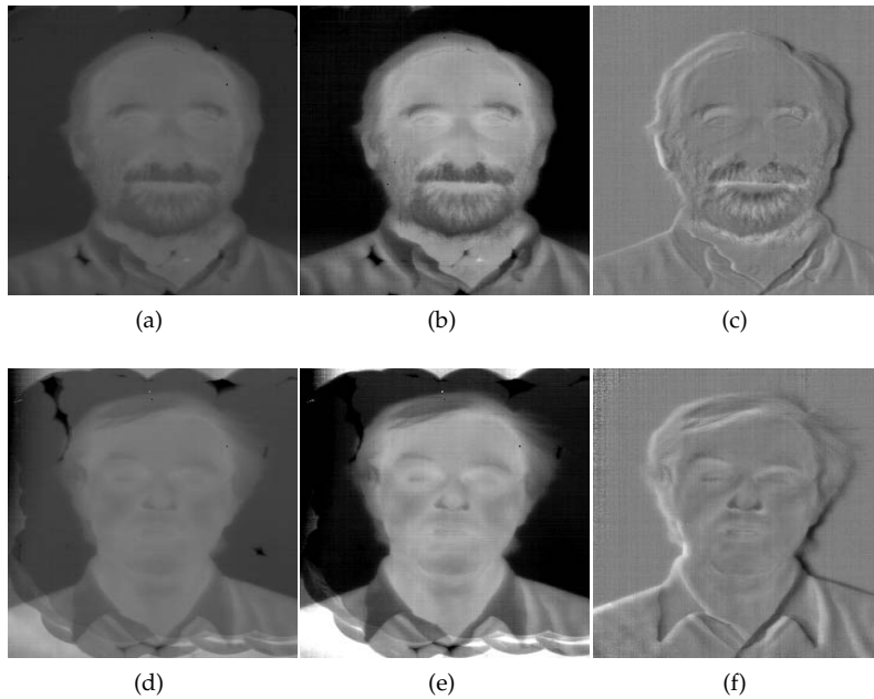
Fig. 5. Full size images of subject 2417 (a) and 2434 (d) from Equinox (2009) database. (b)(e) correspond to the spatial offset adjustment and (c) and (f) is with FPN removed. Its clear that the quality of the images are improved maintaining the 320x240 original spatial resolution.
